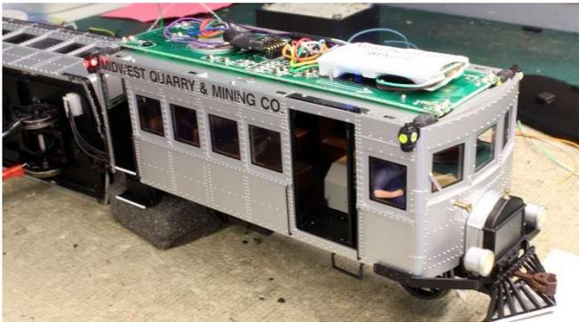
Almost finished, using the wheels on the trailing unit to get power to the loco for programming. The marker lights and the interior lights are on the same circuit so they come on together. To separate them would require making a new board and components. With the change of resistors the headlights are better now.
