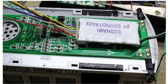
I used double side tape (the Black kind) to hold the decoder in place as shown. I fits nicely in place. This is the ECO 200 – UK but the ECO 100 – UK is smaller and fits well.
